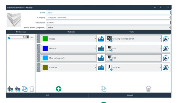
If you are using a **custom** material click on the to add a new method and select 'Thrucut regmark' from the drop down list.
