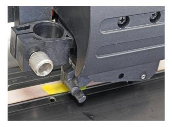
8. Bend the filter up and stick the end of the filter to the housing of the OPOS sensor.
