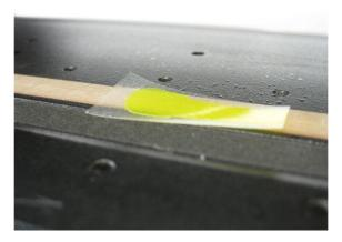
**4.** Move the cutter head above the filter until the widest part covers the OPOS optics.
