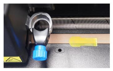
5. Move the OPOS sensor on the cutter head above the wide part of the yellow filter.
