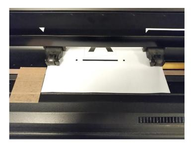
After the pinch rollers were lowered to the media, the machine will skip searching for the pinch roller position, as it assumes all sheets having the same design are of the same size.
