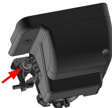
Check knife depth (knife pressure) and knife offset before performing the tests.
