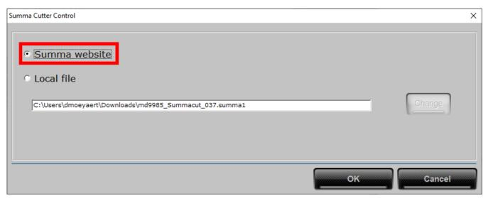
In case the firmware upgrade file was already downloaded, then select [Local file] and click on [Change] to navigate to the folder where the downloaded upgrade file firmware was stored, and select the new firmware:
