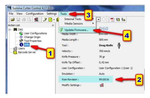
In case the ROM Revision is lower than 9910016, and you want to use the USB port, it needs to be upgraded in order to be used with Windows 8 or 10. You must then use the serial port to perform this upgrade in case this has to be done from a Windows 8 or 10 computer.
