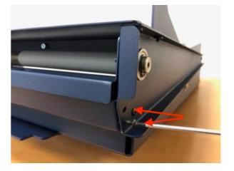
Loosen the 3 nuts. You are now able to adjust the height of the separator.
