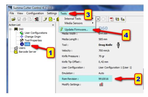
In case the ROM Revision is lower than 9910 016, and you want to use the USB port, it needs to be upgraded in order to be used with Windows 8 or 10. You must then use the serial port to perform this upgrade in case this has to be done from a Windows 8 or 10 computer.
