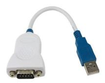
In case the cutter is connected to the computer using a USB-RS232 adapter, the USB driver for this adapter needs to be installed (and not the one from Summa), and in Summa Cutter Control, the serial port this adapter is emulating should be selected. You will also need to use the serial cable delivered with the machine (reference 423-183) to connect the adapter to the cutter.
