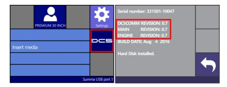
The firmware version of the machine can also be checked from Summa Printer Control.
