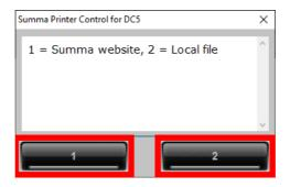
Click on [1] to have Summa Printer Control downloading the right firmware, or click on [2] to use the previously downloaded firmware, and select the firmware:
