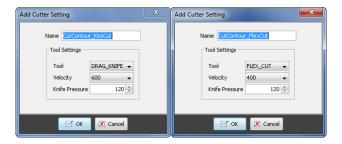
It is convenient to add to two layer settings. One for Kiss Cut and one for Cutting Through (FlexCut). The Names should be exactly the same as the spot colours used in the design.
