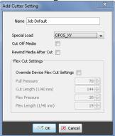
For maximum accuracy of the system set Special Load to OPOS\_XY. Depending on the machine type and driver version extra setting can be made. Close the dialog.
