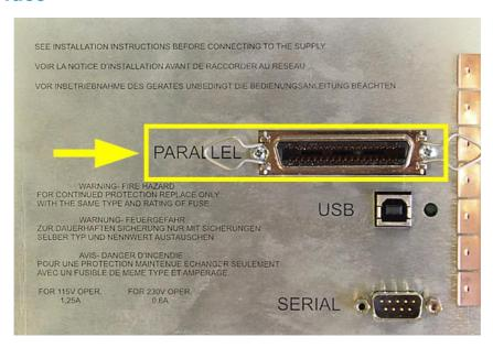
When the cutter is connected using the parallel interface, you do not need a driver, you have to select the correct parallel port in the cutting software.
