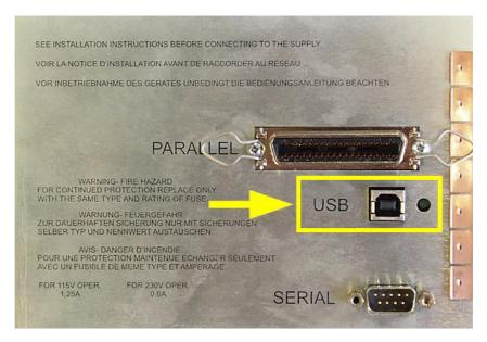
To be able to use the USB interface, a USB driver needs to be installed. This driver is available from the support page of the Summa website:
