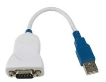
In case the cutter is connected to the computer using a USB-RS232 adapter, the USB driver for this adapter needs to be installed (and not the one from Summa), and in the software driving the cutter, the serial port this adapter is emulating should be selected. You will also need to use the serial cable delivered with the machine (reference 423-183) to connect the adapter to the cutter.
