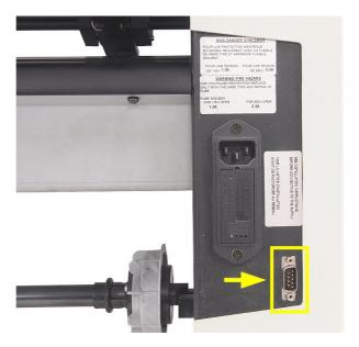
As the cutter is connected using the serial interface, you do not need a driver, you have to set the correct settings in the cutting software.
