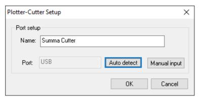
In case the cutters were not yet switched on, or when the firewall prevents auto-detection of networked cutters, then click on [Manual input], and select the communication port to be used.
