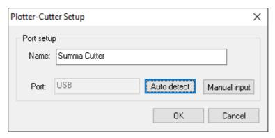
To add multiple cutters, after starting WinPlot, make sure any design in WinPlot is closed. Then click [Design] – [Cutters] – [Install Cutter...].
