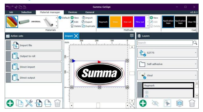
This program can import PDF, DXF, OXF and SGP files and then send data to the cutter. Most design programs are able to generate files in one of those formats.
