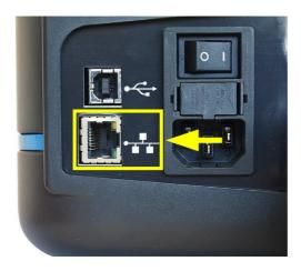
When the cutter is connected using the network interface, you do not need a driver, you have to set the correct settings in the cutting software.
