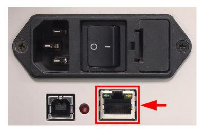
When the cutter is connected using the network interface, you do not need a driver, you have to set the correct settings in the cutting software.
