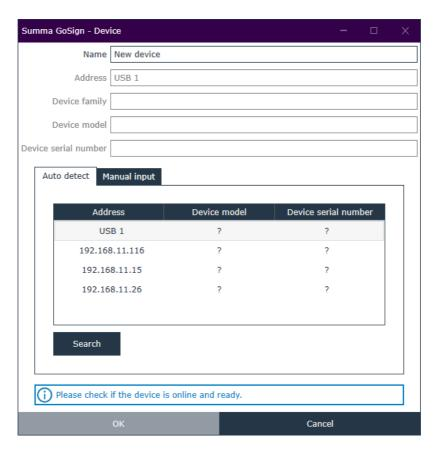
For GoSign to be able to query the info needed from the cutter, media needs to be loaded. Load media in the cutter(s), and click the [Search] button.
