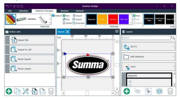
**Note**: The firmware of the machine has to be at least revision 039 to be able to work with GoSign 2.1. In case the firmware is on a lower level, then an upgrade of the firmware is required.
