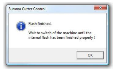
Do not power down the cutter until the cutter displays this to do so.
