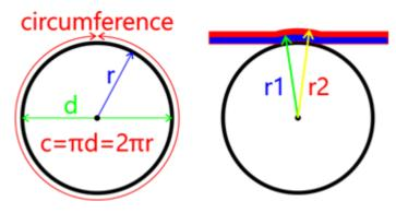
In above diagram, the red colored media is thicker compared to the blue media. The red media will feed further than the blue media for the same amount of revolutions of the drive drum.
