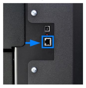
When the cutter is connected using the network interface, you do not need a driver, you have to set the correct settings in the printer-cutter and Summa ColorControl.
