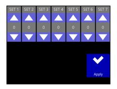
is cut on top of the printed test pattern. Check for the squares where the cut line is situated just above the printed line. Use those values to insert via the control panel. If the values were too far off, then use the best matching value, and then redo the test.
