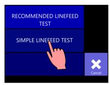
The linefeed test is printed in the OptiTrac color selected previously (e.g. cyan). The "Recommended Linefeed Test" combines the "Media Calibration" test followed by the "Simple Linefeed Test".
