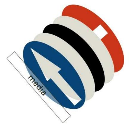
You can see that on top of the media a blue layer is printed followed by a white one, black one, white one and finally a red layer. The combination of this will give the impression that the red stop sign has been printed on a white opaque material as will the blue go sign.
