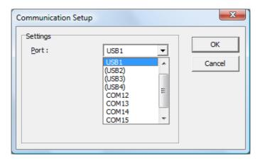
USB-ports listed between round brackets are not available, usually because the cutter was not connected using the USB interface and/or powered on, or was not configured for the listed USB port.
