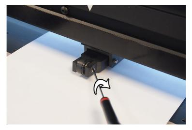
Push the shaft out of the pinch roller block.
