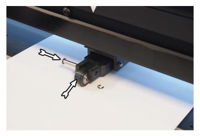
Position the clip on the shaft and push down.
